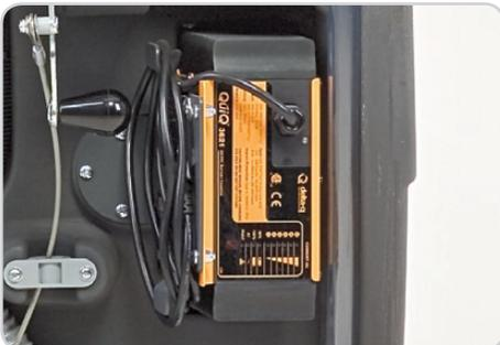
Warrior™ AXP™ scrubber includes a standard onboard battery charger for wet or gel battery packages.
