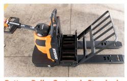
Battery Roller System is Standard Saves time and effort during battery change-outs
