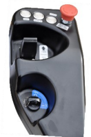
Travel, Lift, Lower, Key Switch and EPD Controls
